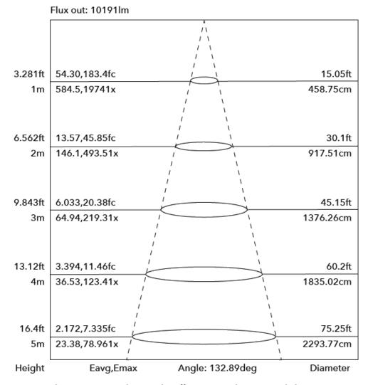
Note: The Curves indicate the illuminated area and the average ilumination when the luminaire is at different distance.
