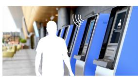
Motion is detected and a timer starts When motion is detected a 15 second timer begins. The sensor will reset the timer and the device will not turn on while anyone is still within range.
